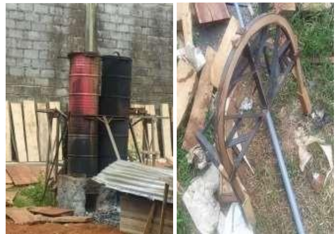
(a) Gambar 2. (a) Drum Boiler Steam Kayu, (b) Cetakan Lengkungan Kayu
